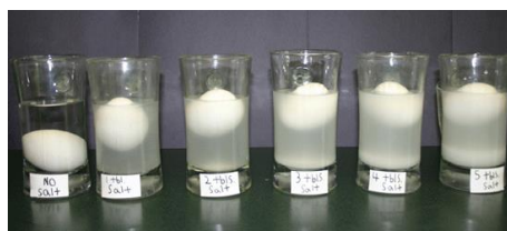
Figure 2: buoyancy experiment with eggs. Picture taken from http://physics.stackexchange.com/questions/59962/how-dense-fluid-affect-the-buoyancy-force .
